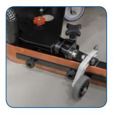
operator's misuse. Heavy duty V-shaped squeegee ensures perfect drying of every type of floor, even with large joints. Nonmarking wheels avoid marks after the drying. Completely adjustable to fit any surface.
